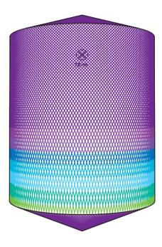
D8m H10m, Toftejorg TZ-66, 4 x  $\emptyset$ 10 mm, 0% Time = 23.3 min., Water consumption = 10868 I
