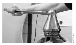
11. Check that the turbine assembly can move freely in the top part assembly
