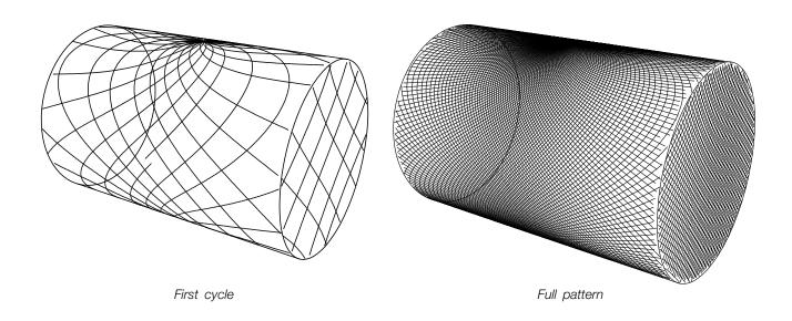
The number of cycles needed to perform a proper cleaning depends on type of soil, distance between tank cleaning machine and tank wall, cleaning procedure and cleaning agent. For residues that are easily mobilized, i.e. easy to remove, one cycle could be sufficient. Heavier soiling (high viscous, sticky substances, etc.) requires more cycles (a denser pattern).
