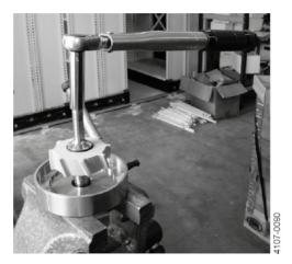
5. Screw the shaft end (3.4) into the turbine shaft (3.1) using the torque wrench (TE81B156) and NV9 spanner socket (TE81B158). Tighten with torque of 10-12 Nm.
