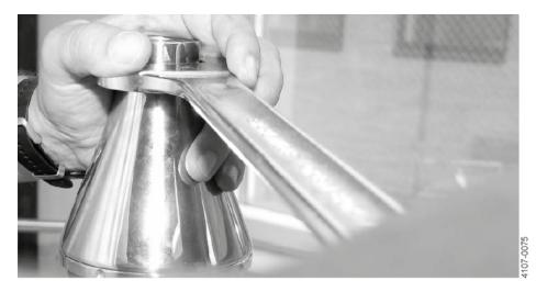
4. Loosen the cone (1.1) by hand while lifting the cone vertically and finally remove the cone (1.1)
