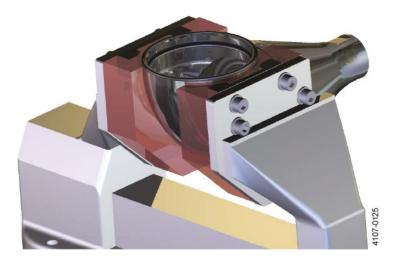
16. Preparation before mounting the assembled lower parts on body (13.1): It is recommended to grease the body thread with food graded/FDA compliant grease. The grease reduces the risk of galling in threads. The grease is enclosed between the O-rings and, therefore, it will not come into contact with the cleaning media.
