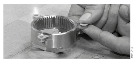
2. Mount bearing for body (13.3) on the gear frame (13.2). Use Drift (TE81B139) and hammer to apply pressure.
