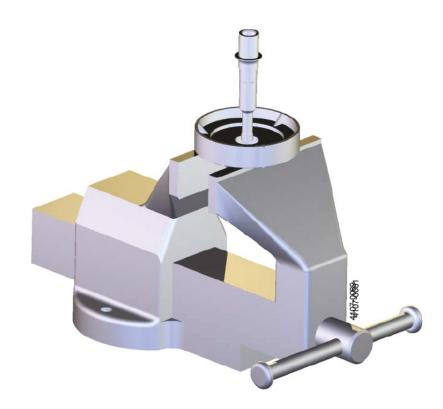
4. Place impeller (3.2) with O-rings (3.3) onto the impeller shaft
