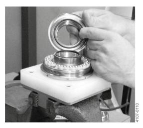
10. Screw the bevel gear (14) on to the nozzle head (18) thread by hand
