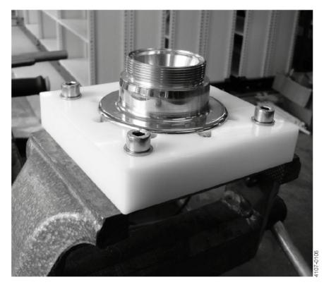
3. Lower the hub nut (15) vertically around the nozzle head (18).
