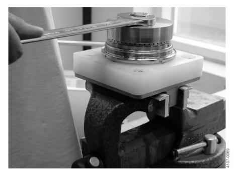
4. Remove the bevel gear (14), the O-rings (16 and 17) and the ball race (5 – identical with the one used around the stem)
