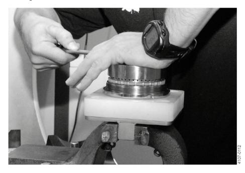
12. Check that the hub nut (15) can rotate freely and that O-rings inside are mounted correctly (16 and 17).
