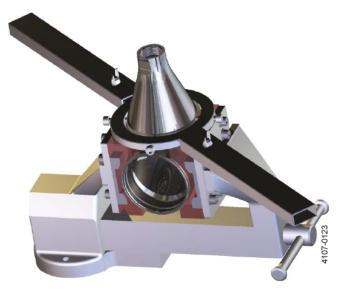
11. Tighten the stem nut (4) until you feel a stop and then tighten a bit more (the stop you feel are two surfaces connecting).
