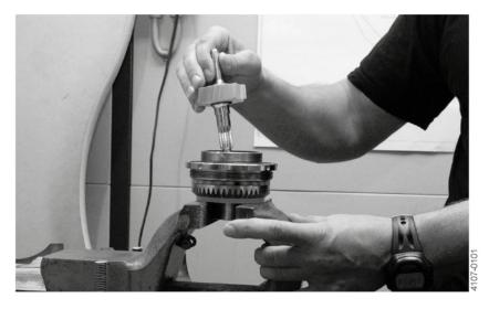
9. Carefully screw the cone (1.1) onto the stem (8) by hand.
