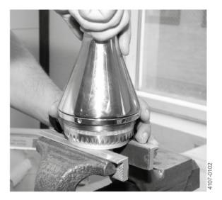
10. Tighten the cone (1.1) using the ring key spanner (TE81B141 or TE81B159) until you feel a stop and then tighten it a bit more. The stop you feel is two surfaces connecting.
