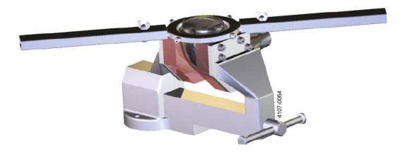
13. Remove hub nut (15) from body. Lift vertically.
