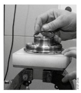
6. Preparation before mounting the bevel gear (14) on nozzle head (18): It is recommended to grease the nozzle head thread with food graded/FDA compliant grease. The grease reduces the risk of galling in threads. The grease is enclosed between the O-rings and, therefore, it will not come into contact with the cleaning media.
