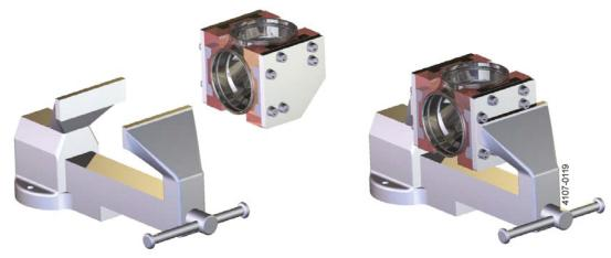
2. Mount assembled gear ring in body (13.1). Tighten screws (13.5) using the torque wrench (TE81B156+TE81B157) to maximum 5 Nm. Too much torque breaks the screws.
