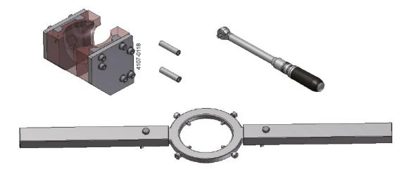
1. Put the two fixtures (TE20J386) around the house and slide the assembly between the jaws of the bench vise. Let the bolt ends slide on-top of the jaws. With the SaniJet 25 centred between the jaws tighten the bench vise.
