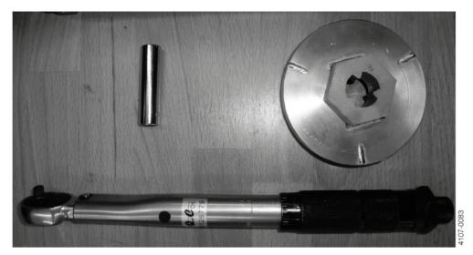
1. Mount the impeller turbine fixture (TE20J392) in bench vise. Loosen the shaft end (3.4) using the torque wrench and NV9 socket long (TE81B156 + TE81B158) and unscrew with hand.
