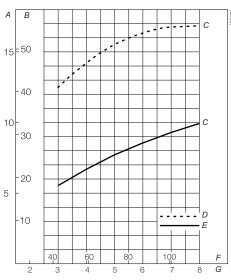
Inlet pressure A: m. B: ft. C: All nozzle sizes. D:max. static. E: Effective. F: psi. G: bar
