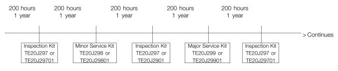
It is recommended to inspect the Alfa Laval Toftejorg SaniJet 25 after every 200 running hours or after 1 year to ensure the conditions of the machine is acceptable. During the inspection it is recommended that the inspection kit is used in order not to compromise the hygienic state of the machine.
