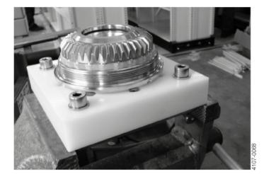
3. Put the hub tool kit (TE20J392) on top of the bevel gear (14) and loosen the bevel gear using ring key NV36 (TE81B159).
