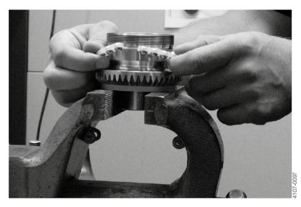
4. Place the stem nut (4) onto the stem (8), while keeping the stem horizontal. Do not apply any force to it.
